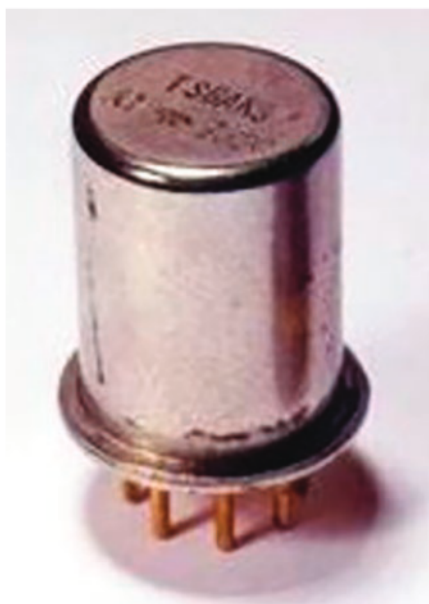
Reproduced rather significantly larger than life size, this is the TS6AK5 used in the Fetron Receiver. The type number is designed to show its equivalence to the 6AK5 valve.
