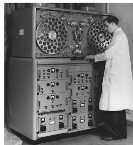
The BBC's Video Electronic Recording Apparatus (VERA) was an attempt to record video onto tape in a similar manner to audio. It used stationary heads and a very high tape speed, necessitating huge tape reels. Despite their size, each reel only lasted 15 minutes! Source: www.vtoldboys.com
